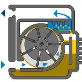
remarkable advantages, first among them being **greater volume yield** because <sup>7</sup> the vanes are in constant contact with the inner wall of the stator and form a perfectly airtight seal with no leaks along the wall thanks to a continuous film of
