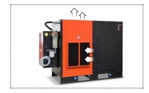
Cooling is an important factor during the compressed air production process, as it helps to increase system efficiency and reliability. **The new Blade 8-12 is equipped with an electric fan with an integrated inverter.** The rotation speed of the cooling fan adapts itself to the working conditions and the environment, optimizing performance and allowing safe operation up to an ambient temperature of + 46 ° C.
