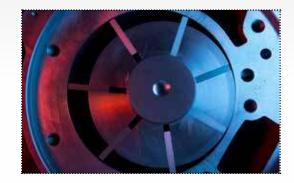
Mattei airends rotate slower than other types of compressors and their blades slide frictionless on a thin film of oil which ensures complete reliability. Mattei machines also have fewer moving parts than other compressors and as the rotor runs on bushes, it has a **virtually unlimited lifespan**.
